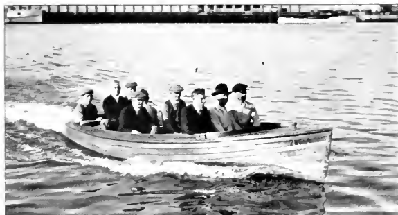
An 18-foot family launch. This is another Fellows &amp; Stewart standard type. Powered with a 12 horsepower Universal engine, she makes easily 10 miles an hour when fully loaded.
